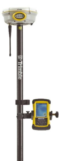
The Trimble® 5800 Limited GPS System is a surveying system that combines a dualfrequency GPS receiver, antenna, UHF radio, and battery in a single compact unit.
